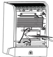
4. Gently insert the Purifier Plate between the guides (inside the cage) until it stops.
