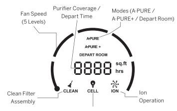
Flicker: Replace ActivePure\* Cell Red Light: ActivePure\* Cell Malfunction
