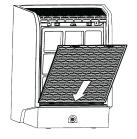
5. Replace the Filter Assembly, inserting the bottom of the Filter Assembly first.
