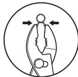
3. Slide each hose clip to about 1/8" of the tubing end to secure the tubing to the barbs.
