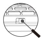
2. Use the included screwdriver to secure the Filter Assembly.
