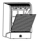
3. Lift up to remove the back panel
