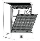
3. Place the Back Cover on by inserting the bottom of the Back Cover first.
