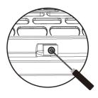
5. Use the included screwdriver to screw in the Filter Assembly.
