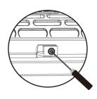
Use the included screwdriver to unscrew the Filter Assembly.
