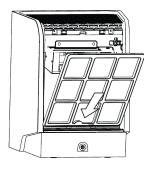
4. Replace the Filter Assembly, inserting the bottom of the Filter Assembly first.
