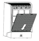
Place the Back Cover by inserting the bottom in first and snapping into place.
